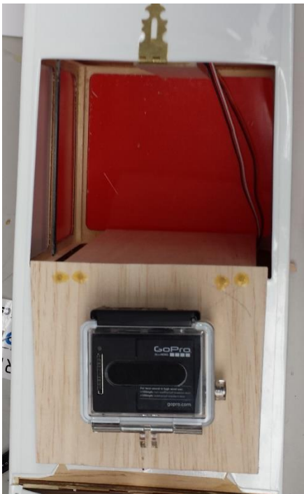
Figure 20 - Open Camera Mounting Hatch with Excavated Aircraft Cavity
